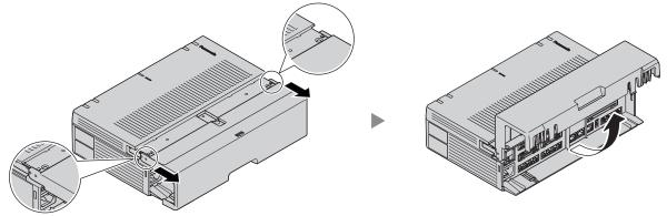
**2.** Holding the cable cover open at about a 90 angle, remove the cable cover by pushing it in the direction of the arrow as shown below.
