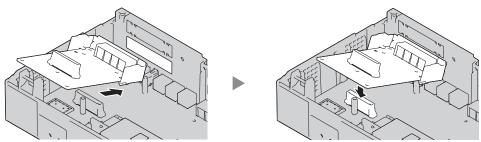
**3.** Insert the spacers (①) into the holes on the card, and tighten the spacers to secure the card.
