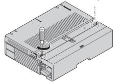
3. Slide in the cable cover and turn the screws clockwise to tighten them. Then, close the screw cover.
